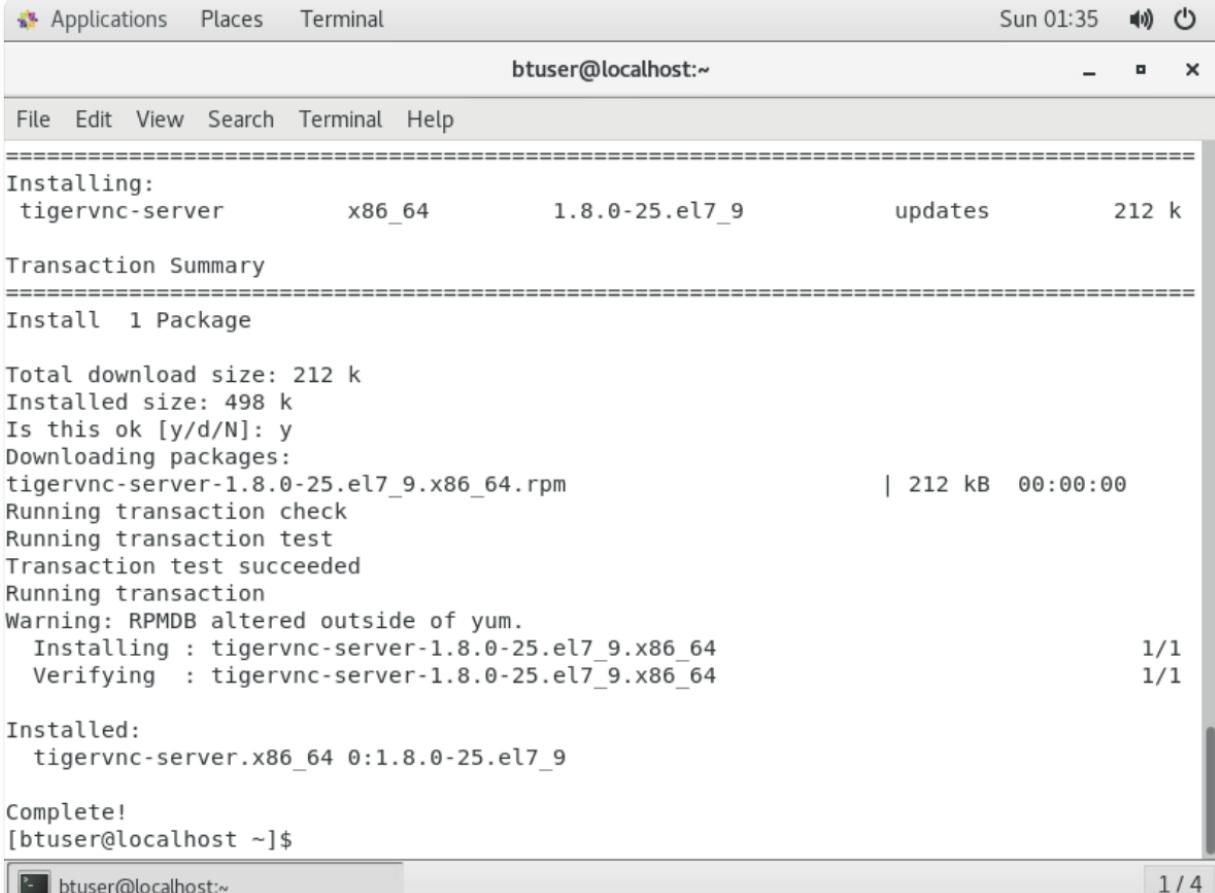
A screenshot of a terminal window titled "btuser@localhost:~". The window shows the output of a yum install command for the "tigervnc-server" package. The output includes the transaction summary, package download, transaction check, test, and final verification steps. It ends with a "Complete!" message.
